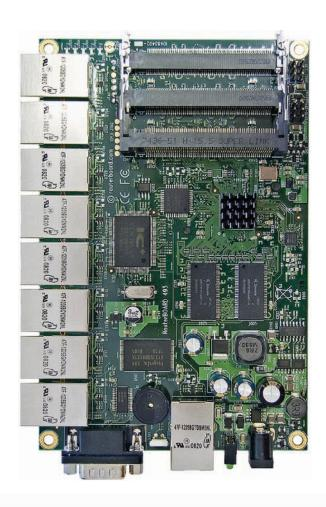
The RB493AH has nine ethernet ports and three miniPCI slots, it also has a switch chip, so the ethernet ports of your choice can be grouped together to make it act as a switch.
